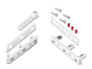
The tappet contacts ST9131 (white) and ST9132 (black) are suitable for transmission of electricity to windows or doors. A permanent electrical contact stability is ensured by a strong magnet that attracts the magnetic tappets. This contacts work entirely without access ramp, which allows the contacts to close from each position and side. As a result, the contacts are qualified for both normal window, turn/tilt doors as well as for lifting/sliding doors.
